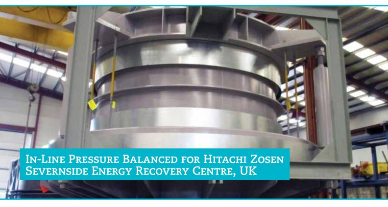
An In-Line Pressure Balanced MPB-I DN 3100 expansion joint has been successfully designed, manufactured and tested for the Hitachi Zosen Inova 34 megawatt energy recovery facility in South Gloucestershire, UK.
